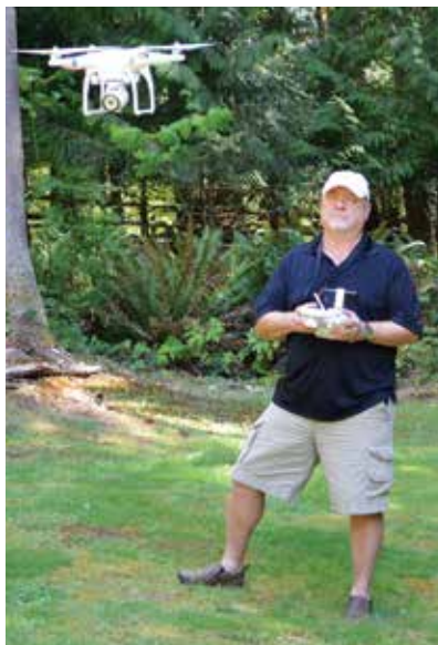
The DJI Phantom 2 Vision quadcopter (above) is equipped with a 14MP camera. A free app live streams what the camera sees to a smartphone (above right) and allows the user to control the camera's angle while it's in flight.
