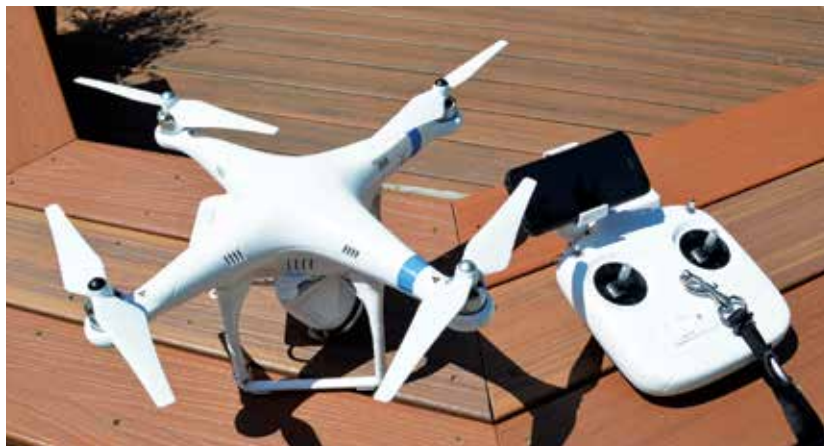
The DJI Phantom 2 Vision quadcopter (above) is equipped with a 14MP camera. A free app live streams what the camera sees to a smartphone (above right) and allows the user to control the camera's angle while it's in flight.
